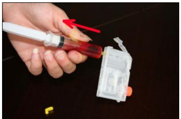
Draw the plunger and do not loose hand for about 10 seconds.
