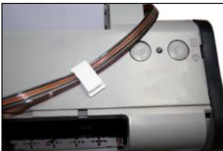
Place the tube through supporting arm. Move the cartridge car to left end and right end. Make sure that the tubes are not too tight or too loose.
