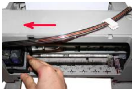
Place the tube through supporting arm. Move the cartridge car to left end and right end. Make sure that the tubes are not too tight or too loose.
