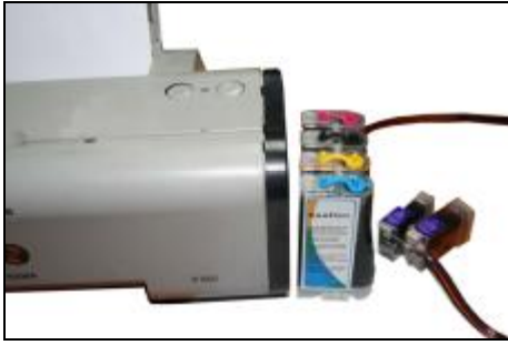
Put the CISS on the right side of the printer. And place all the tubes at correct position.
