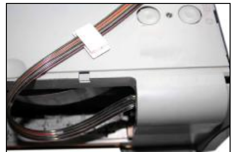
Place the tube through supporting arm. Move the cartridge car to left end and right end. Make sure that the tubes are not too tight or too loose.
