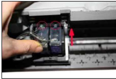
Remove the cartridge bottom cap. And put the CIS cartridges into cartridge Carriage.
