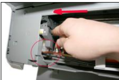
Move the cartridge car to both sides. Make sure that the tubes are not too tight or too loose.
