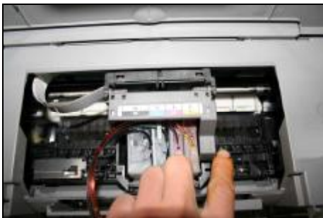
Remove the bottom cap from CISS cartridges. Place them into cartridge carriage carefully. Fix the support arm, which should be 4 cm from the right edge of printer, place the tube through supporting arm as the picture shown above.
