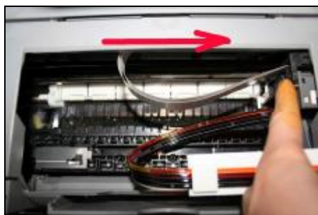
Move the cartridge car to both sides. Make sure that the tubes are not too tight or too loose.
