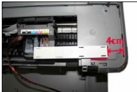
Remove the bottom cap from CISS cartridges. Place them into cartridge carriage carefully. Fix the support arm, which should be 4 cm from the right edge of printer, place the tube through supporting arm as the picture shown above.
