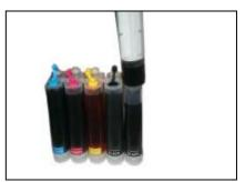
Refill ink according to the color carefully And clean the ink tanks after refilling.
