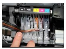
Then put the CISS cartridges into printer
