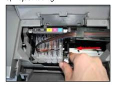
Adjust the tube length and move from Left to right for several times.
