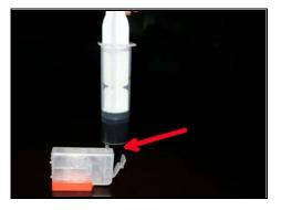
Make sure that the syringe fit the hole very well. Otherwise, Ink could not flow into the cartridge fluently.
