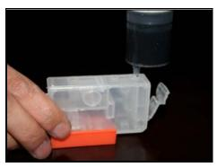
Use the 60ml syringe to draw 20ml ink, then insert it into the refilling hole;
