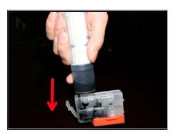
Then loose the plunger, the air pressure will push lnk go into the cartridge naturally.
