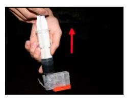
Pull up the plunger for about 15ml to Vacuum the cartridge;
