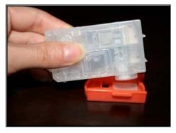
Fasten the cover back onto the cartridges Please make sure it is sealed very well.
