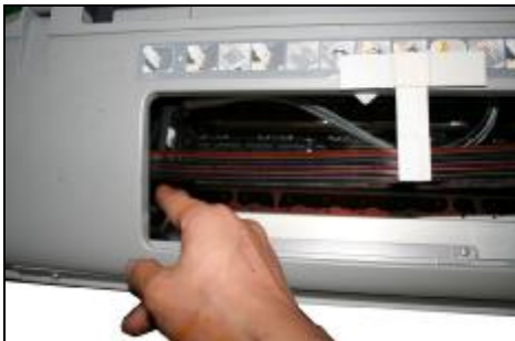
Adjust the tube length and move the carriage car. Insure there's plenty length of tube to make the cartridge cart can horoughly move to the left side.
