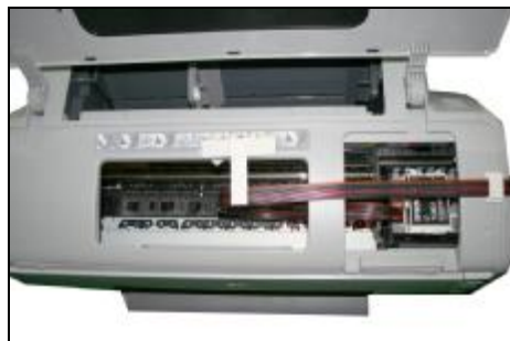
Stimulate the move of the cartridge car. Insure there will no block and when the tubes moving with cartridge car.
