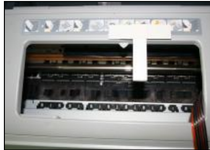
Fix the balance arm on the support arm.
