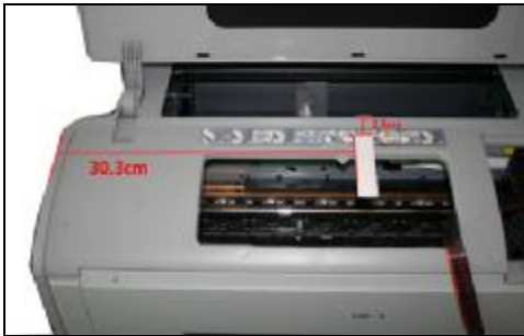
Fit the support arm like the picture shown.
