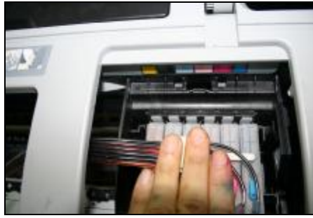
Press those cartridges to make sure it is well installed.
