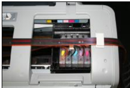
Move the carriage to the right side and make it keeping straight
