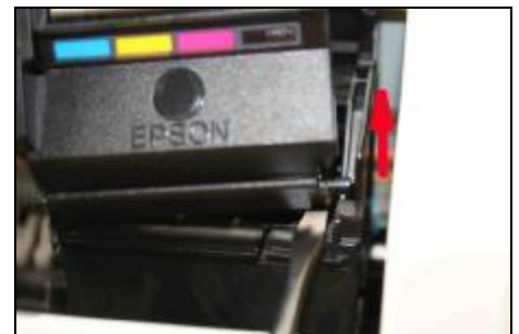
Remove the clip of the cartridge, by circumvolving the screwdriver clockwisely as the red arrowhead shown.
