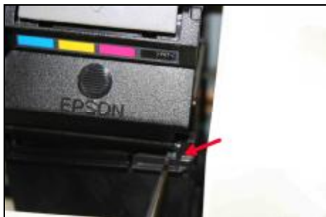
Open up the carriage cover to 60 degree And use a screwdriver to insert into the joint Slightly.
