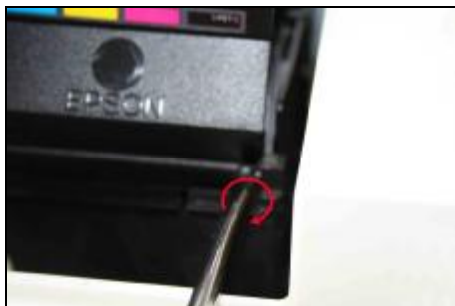
Remove the clip of the cartridge, by circumvolving the screwdriver clockwisely as the red arrowhead shown.
