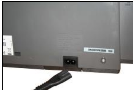
When the cartridge-car to right side, pulling out the power cord.of printer prompt and then you can move the cartridge-car.
