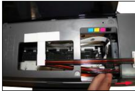
Move the carriage to the rightmost and make sure that the tube can be straight.
