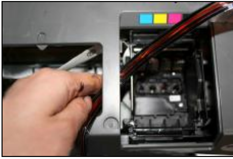
Move the carriage to its original place
