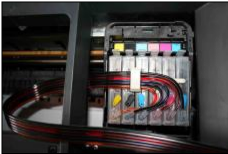
Insert the CISS cartridge in the same way as above picture shown
