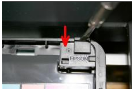
Use a screwdriver to insert into the joint slightly ,
