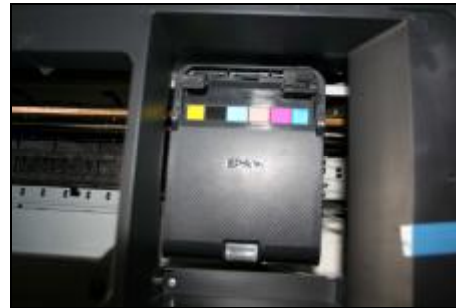
Move the carriage to the right side
