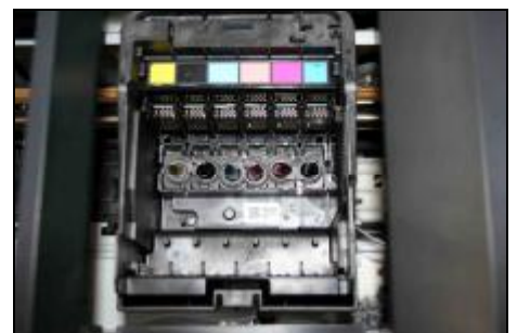
Ready to install CIS
