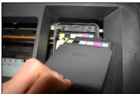
Then remove the cartridge cover directly
