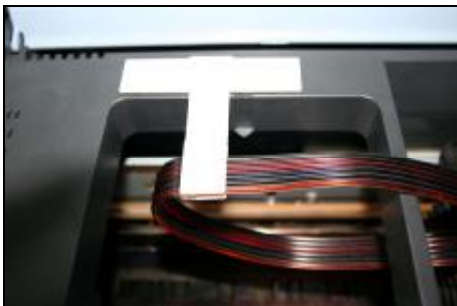
Fix the tube line on the tube holder like the picture shown.
