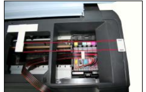
Stick the clip on the right side of the printer, make the tube and the printer in the parallel line.
