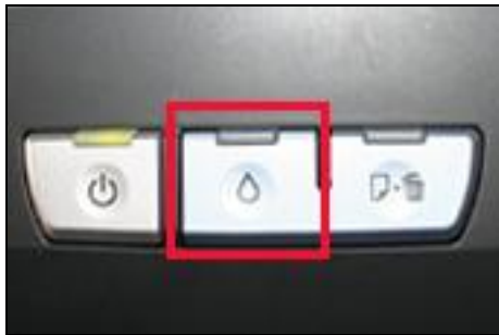
Press the button to replace cartridges
