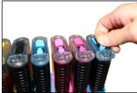
Pull out the small rubber plug from the air hole as picture shown above.
