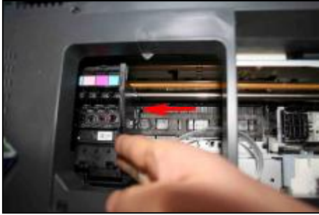
Move the carriage to the left-side
