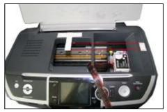
Stick the clip on the right side of the printer, make the tube and the printer in the parallel
