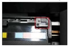
Remove of the cartridges by take off the clips On the carriage.
