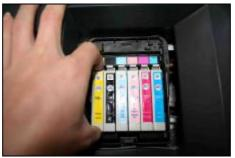
Take out the original cartridges from the printer. Then prepare to install the CIS.
