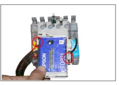
Press cartridge down until it is locked by the circled clips.
