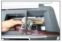
Put in the CIS cartridges as the picture shows. Move the carriage back to its original position.
