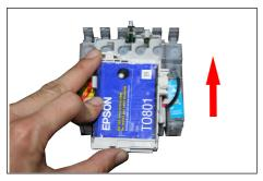
Push it upside until springs fitted with original cartridges completely.
