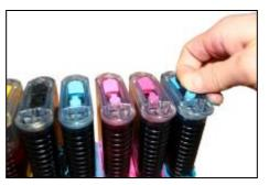
Pull out the small rubber plug from the air hole as picture shown above.
