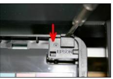
Insert the screwdriver in the aperture slightly as the red arrowhead show.
