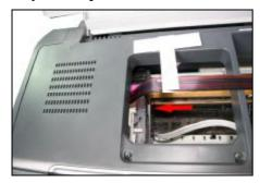
Adjust the tube length and move the cartridge car. Insure there's plenty length of tube to make the cartridge cart can horoughly move to the left side.
