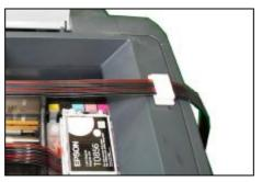
Clip the tube line on the tubing holder.
