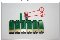
1 reset button. 2 switch. If the switch is turned to up place, then CISS should work with original cartridge. If the switch is turned to down palce, then CISS Can work without original cartridge.
