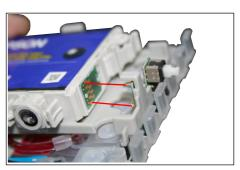
Make sure the top and bottom chip contacts (as picture showing) are well connected. with the two springs on the cover
