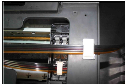
Clip the tube line on the tubing holder.
