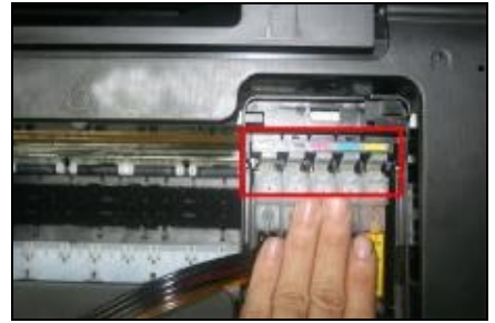
Press the cartridges to make sure it is well installed. You will hear a slight sound when the cartridges are locked well by the clips.
