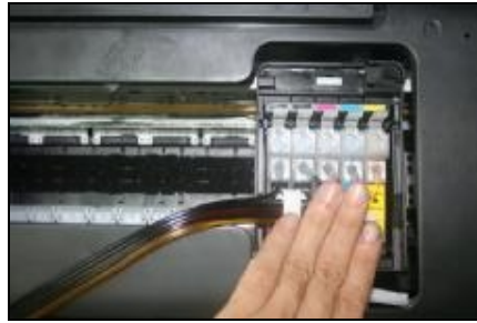
Press the cartridges to make sure it is well installed. You will hear a slight sound when the cartridges are locked well by the clips.
