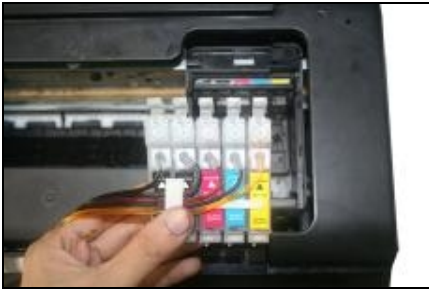
Install the cartridges and match the one-to-one Color.
