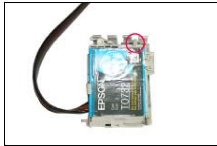
Push it to the top until the third clip locks the cartridge.
