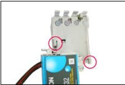
Put the original cartridge on the top of the clips as the red circle showing.
