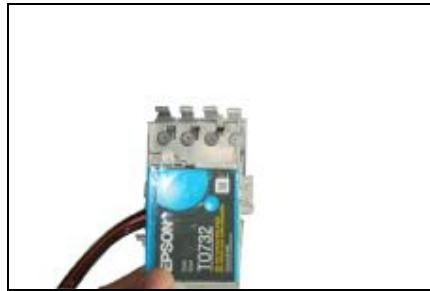
Press the original cartridges to the clips.
