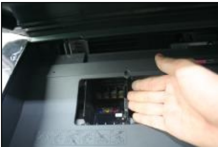
Move the carriage to the left-side
