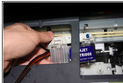
Place the CIS cartridge and pipeline though the printer cover as above picture shown
