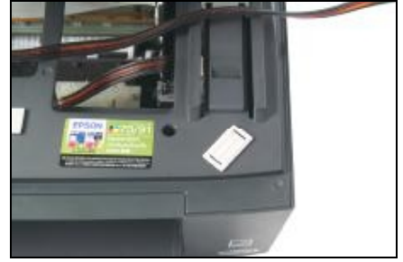
Stick the short support arm parallelly as the above picture shows.
