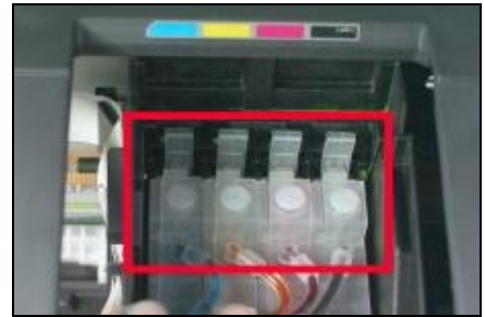
As the red rectangle shown, if all the cartridges are well installed, you can hear some sound.
