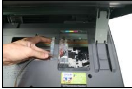
Place the CIS cartridge and pipeline through the printer cover as above picture shown
