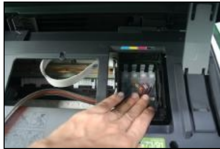
Press those cartridges to make sure it is well installed.
