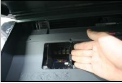
Move the carriage to the left-side
