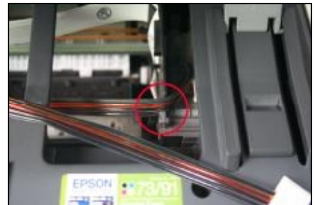
Make sure the tubing pass through the flute.
