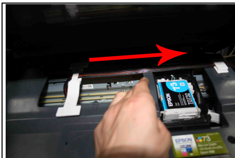
Adjust the tube length and move the cartridge car. Insure there's plenty length of tube to make the cartridge cart can thoroughly move to the left side.
