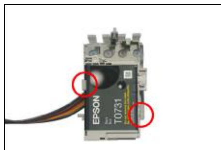
Press the cartridge down until it is locked by the two clips.
