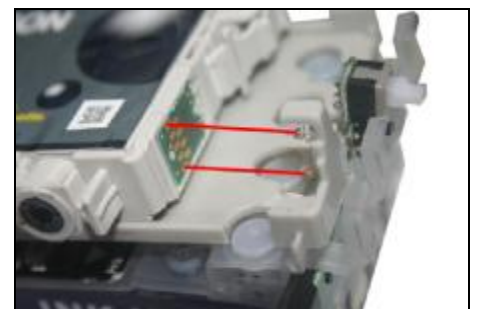
The two metal sheets at the top and bottom Should match the two springs.
