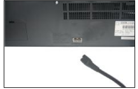
Pull out the power line of the printer and move the carriage to the right side.
