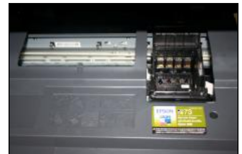
Carriage is empty and get ready for putting in the new CISS
