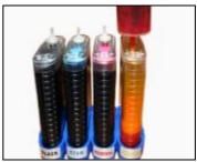
Please kindly to take care of the ink level in the reservoirs, if the ink level is below 1CM from the bottom, it alarms you need to refill the ink duly. Carefully pull out the rubber plugs on the refill holes.(Avoid the ink will spattering out )Refill in the according inkjet ink, wipe the refill hole and rubber plug to keep the clean of it
