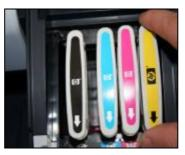
Remove the original cartridges
