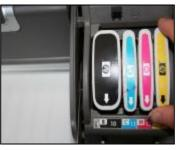
Remove the original cartridges
