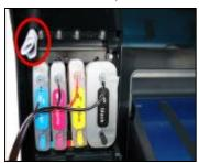
Roll a piece of paper into coniform, Insert it into the small hole which shown in above picture.
