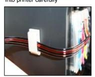
Slightly press every cartridge to check all the cartridges are in the correct position. Please be careful with the tubes which go out from Cartridge Carrier. Then stick the Support Arm on the position which shown in the second & third pictures.
