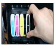
Remove the original cartridges
