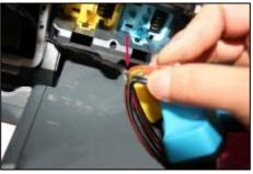
Tear the tubes among the cartridges about 2 cm it will be easier to install the color cartridges.
