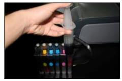
Please pay attention to the ink level in the reservoirs; if the ink level is below 1CM as the above picture shown, please use refill kits to fill ink into Reservoir bottles. Carefully pull out the rubber plugs from the refill holes.(there is possibility of ink spattering. Be careful!) Refill ink according to the color in short supply. Then put the rubber back. (Please keep the printer and the reservoir at the same horizontal line during the process of refilling ink.)
