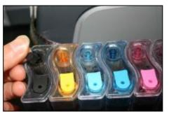
Open the air hole of the inktank.
