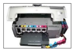
Open the top cover, take out the original cartridges.
