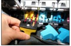
Before you install the CIS cartridges, pls make clear the chip location and make sure that each color cartridge will be installed in the correct location.
