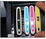
Remove the original cartridges
