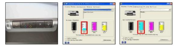
If the indicator light flashing when printing, it tells that you need to reset the chip to full status. Please turn off your printer for about 30 seconds and switch it back on. Ink meter bar shall show full ink. You can start printing as usual.
