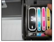
Remove the original cartridges
