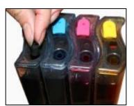
Pull out the small rubber plug from the air hole as above picture shown.
