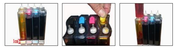
Please pay attention to the ink level in the reservoirs; if the ink level is below 1CM as the above picture shown, please use refill kits to fill ink into Reservoir bottles. Carefully pull out the rubber plugs from the refill holes.(there is possibility of ink spattering. Be careful!) Refill ink according to the color in short supply. Then put the rubber back. (Please keep the printer and the reservoir at the same horizontal line during the process of refilling ink.)
