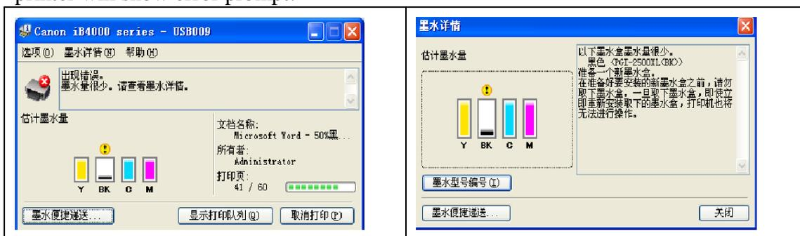
When the printer show this error prompt, you need Turn off the printer,And manually removing the cartridge car, take out the cartridge and fill the ink and install again that can use again. If you keep the cartridge always with ink, will do not show this error prompt.
