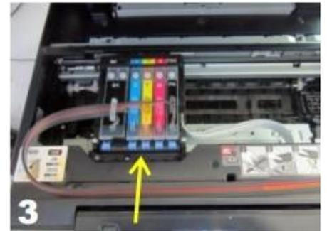
3. Install cartridge into the printer. The cartridge must be install correctly.
