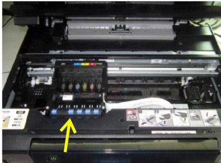
1. Turn on the printer. Perform “change cartridge” operation. The cartridge will move to left as picture show
