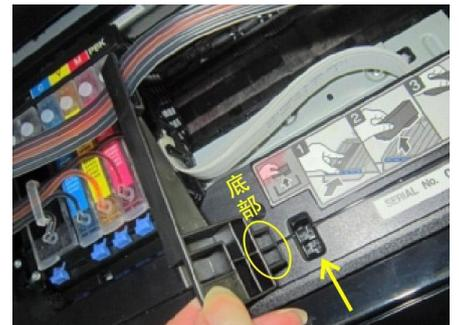
6. Insert the button of support arm on to the place of arrow
