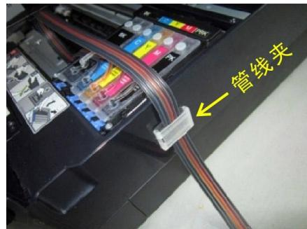
16. fix u support arm, and hold the hose a picture show. Then close the cover of printer. And the printer is ready to printer.
